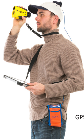
Field-Map Data Collector provides communication with external electronic devices
